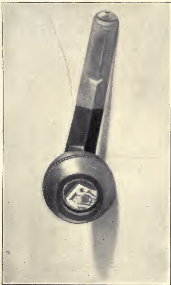
FIG. 22.—PIPE-REFLECTOR IN SITU
